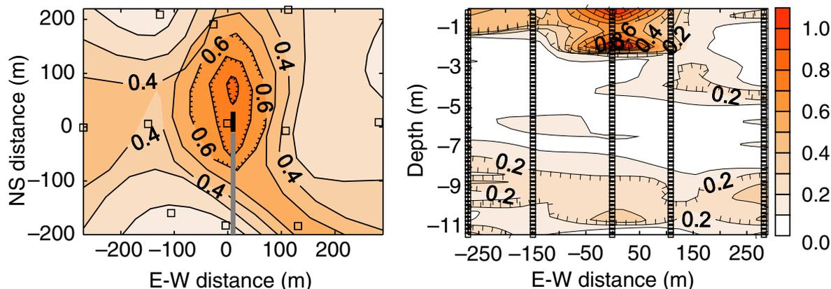
**Fig. 3.** Left: horizontal distribution of  $I_T$  at a depth of 0.2 m on 10 May 2000 above the outfall off Izola. Right: vertical distributions of  $I_T$  in E–W direction that cuts through the central station of the near-field for the respective cruises. Small bars mark the positions where CTD casts were made; dark straight line marks the pipe in a simplified way. [From Malačič & Mozetič (2005), their Fig. 3 (bottom part); with the permission of ACS journals.]
