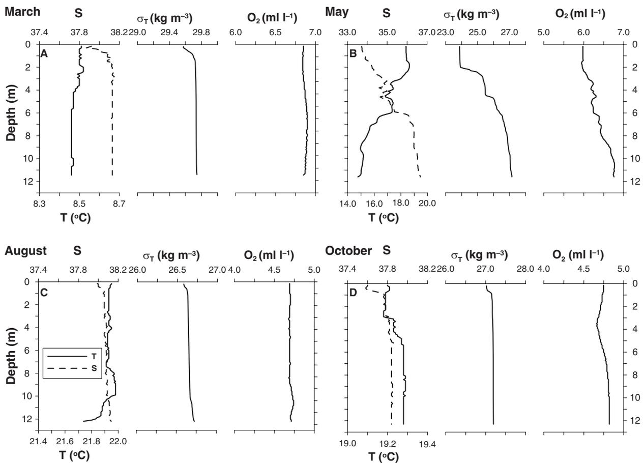
Fig. 2. Vertical profiles of temperature, salinity, density ( $\sigma_T$ ) and dissolved oxygen recorded at station IZ06 during four surveys in the year 2000.
